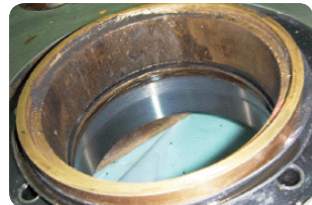
Rod cover damage
